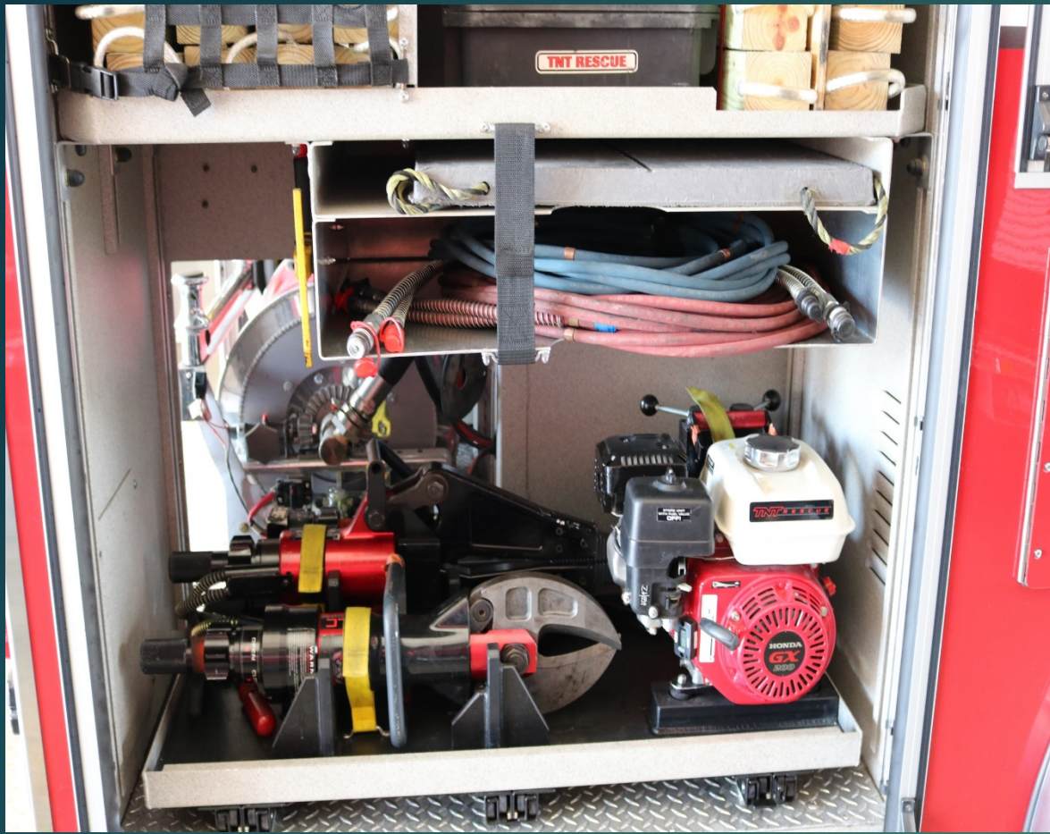
Vehicle Extrication Equipment with power unit And extrication hoses
